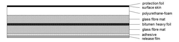
M 1425 is a polyurethane-foam (polyether, thickness 25 mm), surface skin with a grey polyurethane foil, laminated on a composite of two glass fiber mats (thickness 7 mm) with an intermediate heavy foil based on bitumen.
